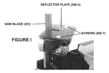
Guide the Saw Blade (251) through the slot in the Vertical Saw Table (55-2), and secure it in position with the two Screws (266-7).
